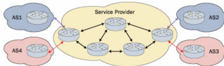
Figure 7. Customer edge-routers in AS1, AS2, AS3, and AS4 can distribute IP VPN routes to Service Provider routers, to reach other routers in other ASs using various tunneling techniques. In BGP/MPLS VPN, multi-protocol BGP is used to circulate VPN routes, and MPLS is utilized to forward VPN packets over the service provider backbone.
