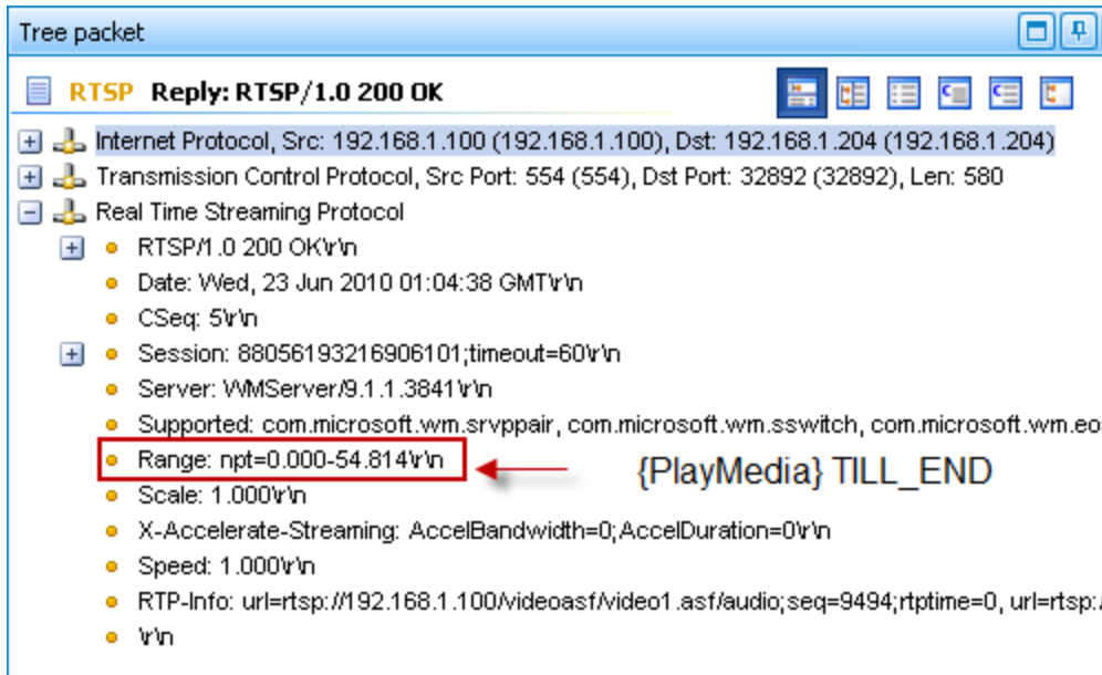
Figure 16. RTSP Describe Response with playback duration information
