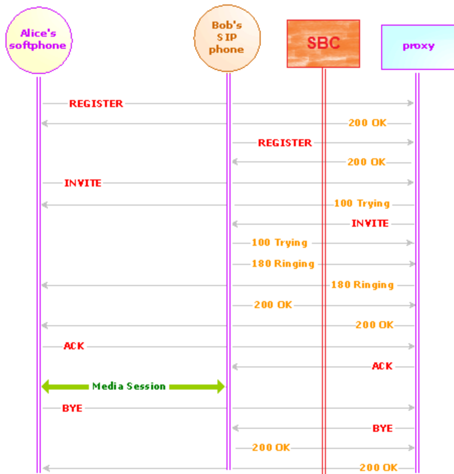
Figure 162. SIP Call flow for Basic Call via a proxy over an SBC
