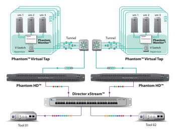
The diagram shows a simple design of traffic flowing from the ESX hosts (and virtual machines) via encapsulated GRE tunnel with a 1/10GB capacity network switch. The Phantom HD appliance (where the GRE tunnel is decapsulated) takes raw data (layer 2-4) and passes it to Director xStream, wherefrom it is regenerated to multiple ports and ultimately fed into the energy provider's AMD instrumentation layer tools.
