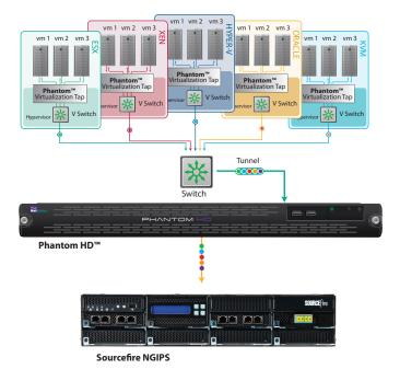
The Phantom tap is deployed in any number of virtual environments to capture inter-vm (east west) traffic. That encapsulated traffic is then sent to the Phantom HD tunneling appliance which decapsulates the GRE header. This traffic can now be inspected by the SourceFire NGIPS for complete security in virtual environment.
