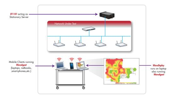
If the test with known good client devices points to the clients, then the system under test (SUT) is the client(s). Use the WaveTest Ethernet WaveBlade or the portable EF1101 Ethernet Test Appliance using the WaveInsite application. A representative test setup is shown below.
