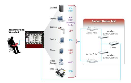
For Step 3 above: The IxVeriWave Ethernet WaveBlade or the portable EF1101 Ethernet Test Appliance, using the WaveInsite and WaveDeploy applications. A representative test setup is shown below.
