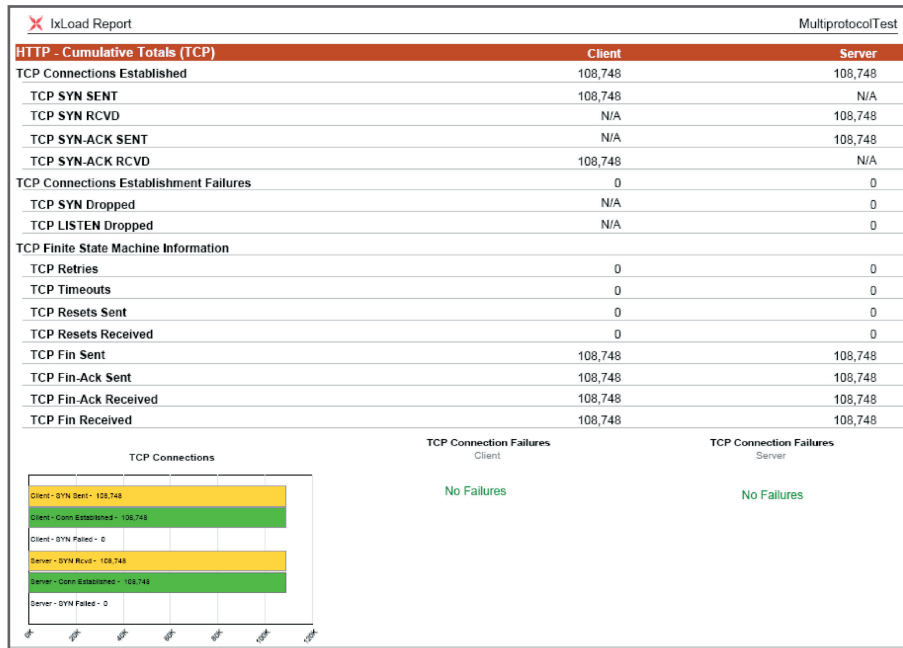
Figure 13. HTTP traffic statistics for the second run with application-layer inspection and IDS engines enabled on the DUT
