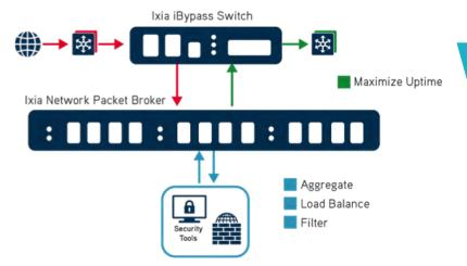
A proper network foundation begins with a stable bypass architecture where inline tools can operate at line speeds without affecting traffic flow in the event of failure.
