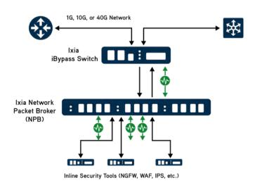
Enable greater scalability and usability from security tools by optimizing load across them and decoupling network link speeds from security tool speeds.
